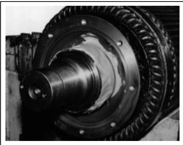
FIG. 16. DRIVE-END INNER BEARING CAP, FLINGER AND BEARING INNER RACE INSTALLED. E-27157.
