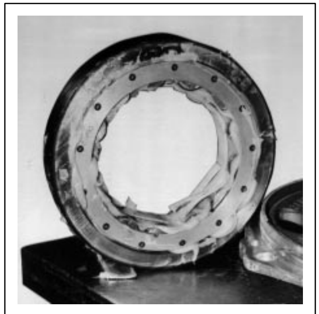
FIG. 18. GREASE IN DRIVE-END BEARING ROLLERS AND OUTER RACE. E-27159.
