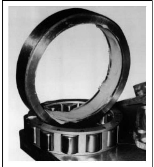
FIG. 17. GREASE IN DRIVE-END BEARING OUTER RACE. E-27158.
